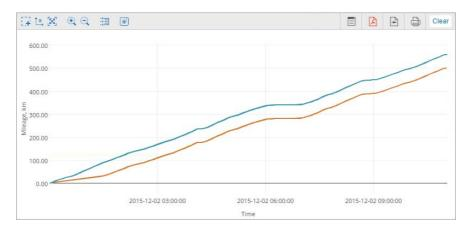
Instant mileage represents data in the form 'mileage from the previous message to the current one' that is the distance between two adjacent messages. This kind of chart can be useful to detect excessive mileage during connection loss, or to detect made-up additions to the mileage.
