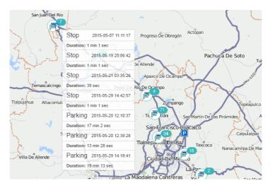
You can enable *Marker numbering* option in report template. In this case, each marker will have its sequence number which is indicated below the marker in red color. Numbers are assigned chronologically, and each marker type has its own numeration.
