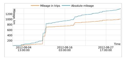
Instant mileage represents data in the form 'mileage from the previous message to the current one' that is the distance between two adjacent messages. This kind of chart can be useful to detect excessive mileage during connection loss, or to detect made-up additions to the mileage.
